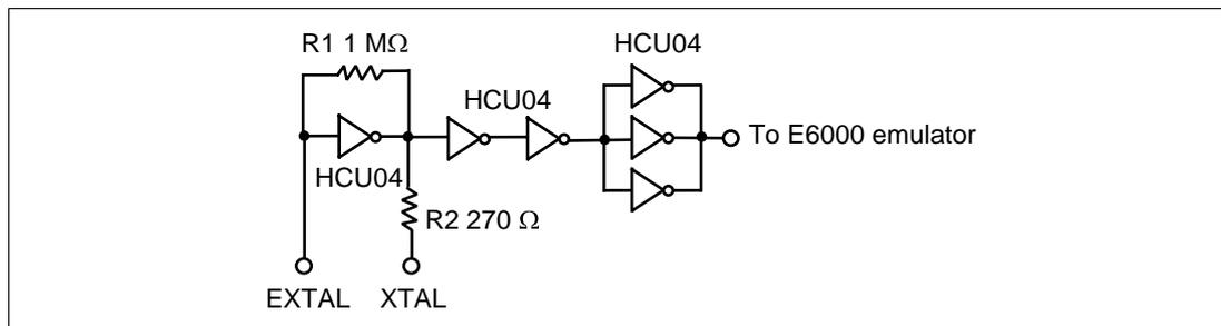
**Figure 9 Oscillator Circuit**
