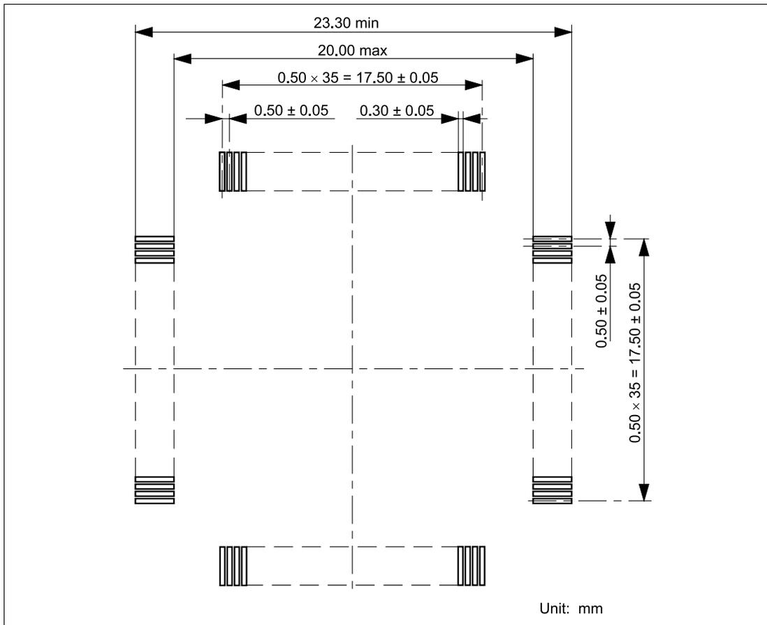
Figure 5 Recommended Dimensions for Mount Pad
