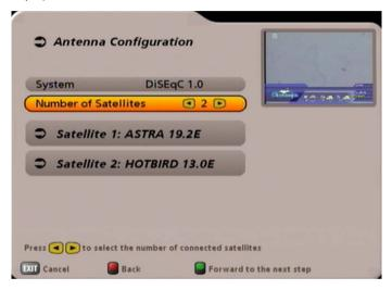
Use the buttons to select the first satellite slot. Press to access the menu for the satellite settings. The following display appears (example):
