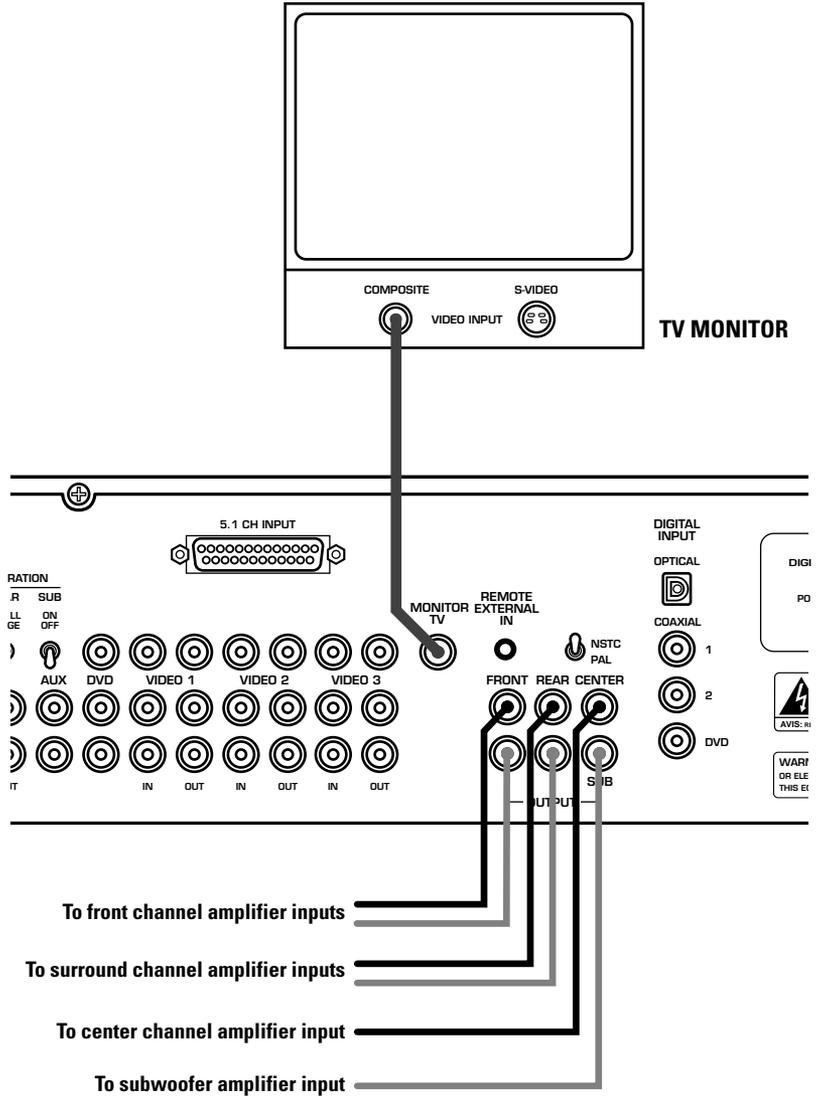
Figure 4: Input Connections
