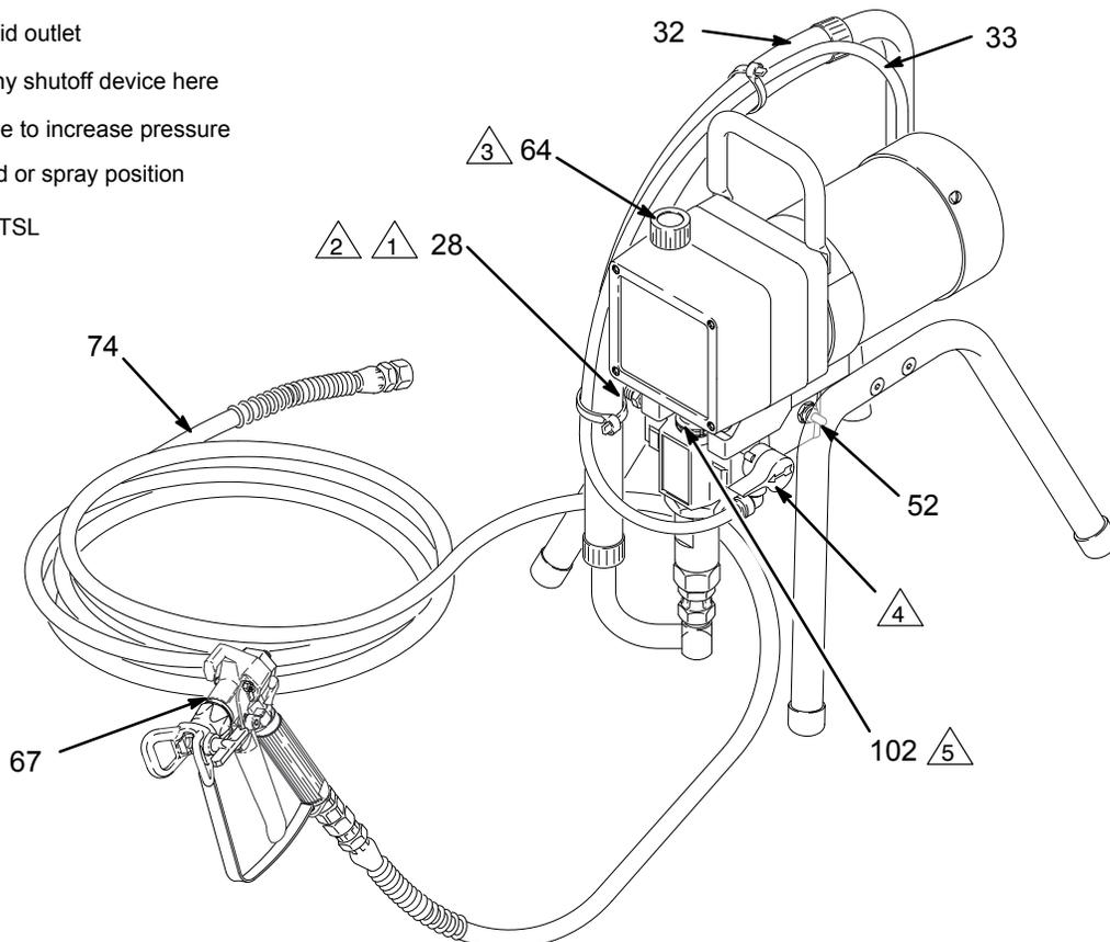
2. **Fill the wet-cup (102).** Pry off the wet-cup seal. Fill the cup 1/3 full with Graco Throat Seal Liquid (TSL), supplied. Install the wet-cup seal.
