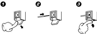
**How to connect AM antenna cord to the main unit**
