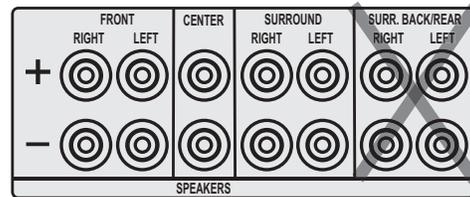
If you have a 6.1 or 7.1 channel receiver, connect the SSA's surround channel inputs to the "Surround" outputs of your receiver, not the "Rear" or "Surround Back" outputs.
