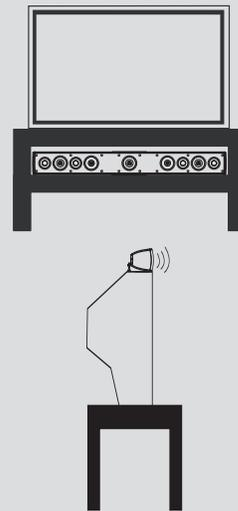
If placed on a shelf under a TV, adjust the leveling feet (screwed all the way in) to aim the speaker up towards the listeners.
