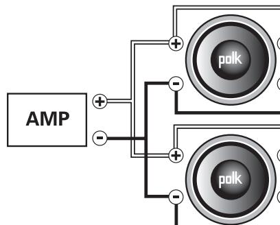
Coils and speakers wired in parallel
