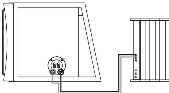
wiring diagram for DXi 1201
