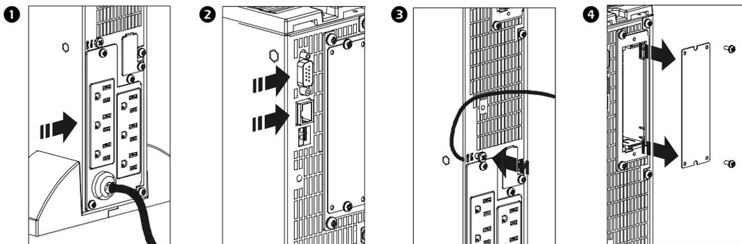
**If Required, Connect the Emergency Power Off (EPO) Feature**
