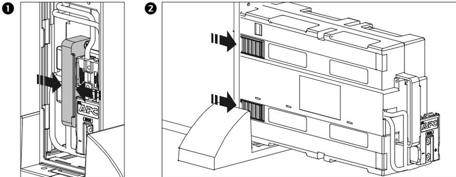
4. Refer to the battery replacement instruction sheet to install the replacement battery in the UPS.
