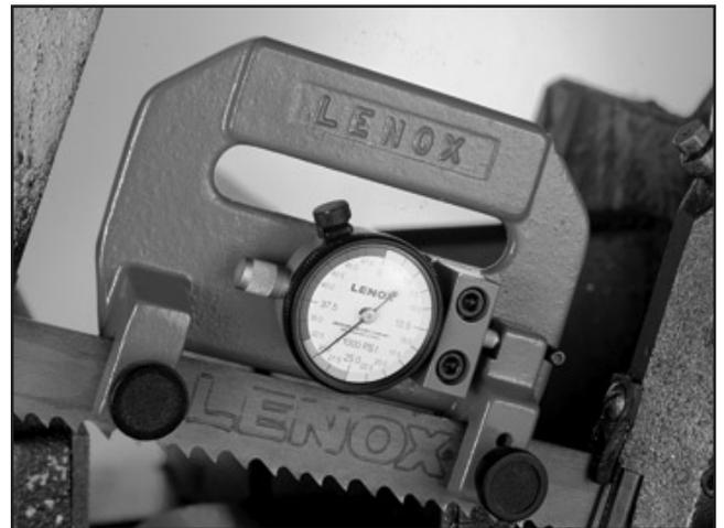
Figure 48. H5408 Blade Tensioning Gauge.
