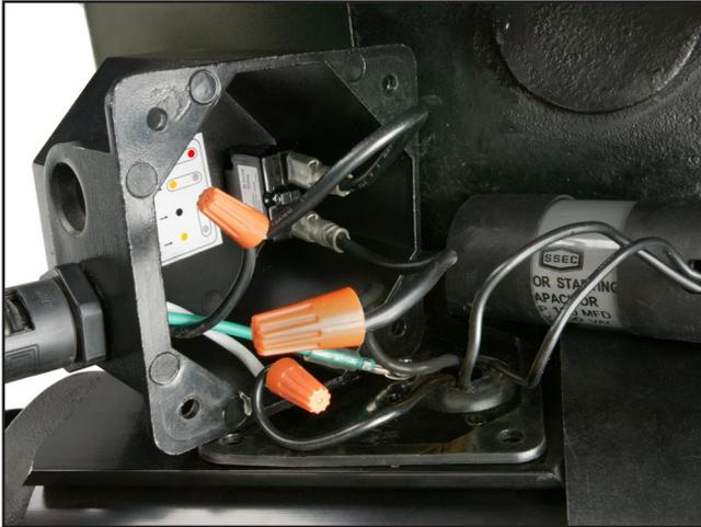
**Figure 61.** Motor junction box wiring.
