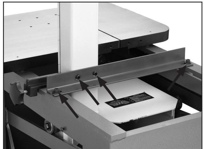
**Figure 8.** Removing shipping bracket.
