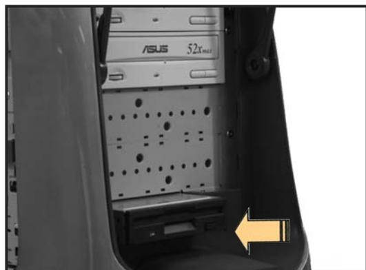
5. Slide the drive bay lock to the left, towards the  $\ominus$  sign to lock the drive bay and to secure the drive in place.
