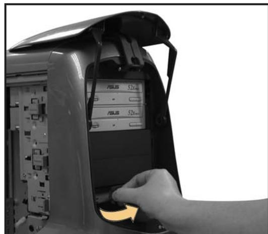
3. Using a screwdriver, push the knock down metal cover in and out of the chassis until it is removed.
