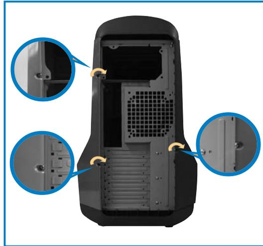
4. Turn the side swivel to about 45° clockwise to release the side panel.
