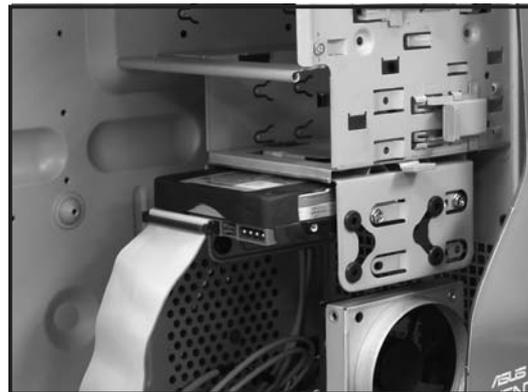
7. Connect a 4-pin power plug from the power supply unit to the power connector at the back of the drive.
