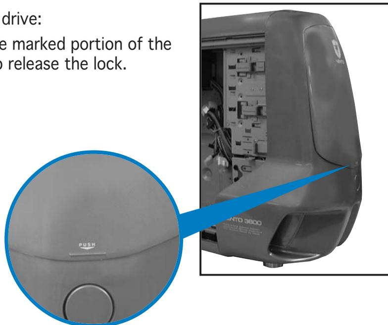
2. The Magic Mask® lifts to reveal the face plates of the drive bays.
