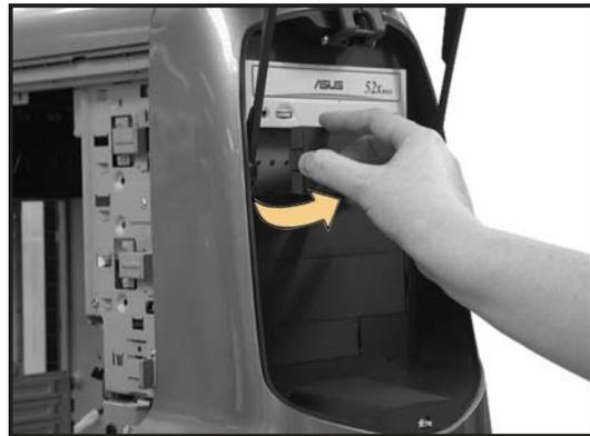
3. Using a screwdriver, push the knock down metal cover in and out of the chassis until it is removed.
