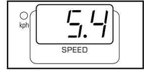
pressed, the speed will change by 0.1 mile per hour (mph). The buttons can be held down to change the speed quickly. The speed range is 0.5 mph to 10 mph. Note: When the SPEED buttons are pressed, the SPEED display will show the selected speed setting for six seconds. The display will then show the actual speed of the walking belt.
