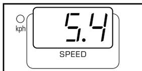
Note: The speed can be shown in either miles per hour (mph) or kilometers per hour (kph). The KPH indicator beside the SPEED display will light when the speed is shown in kph. To change the unit of
