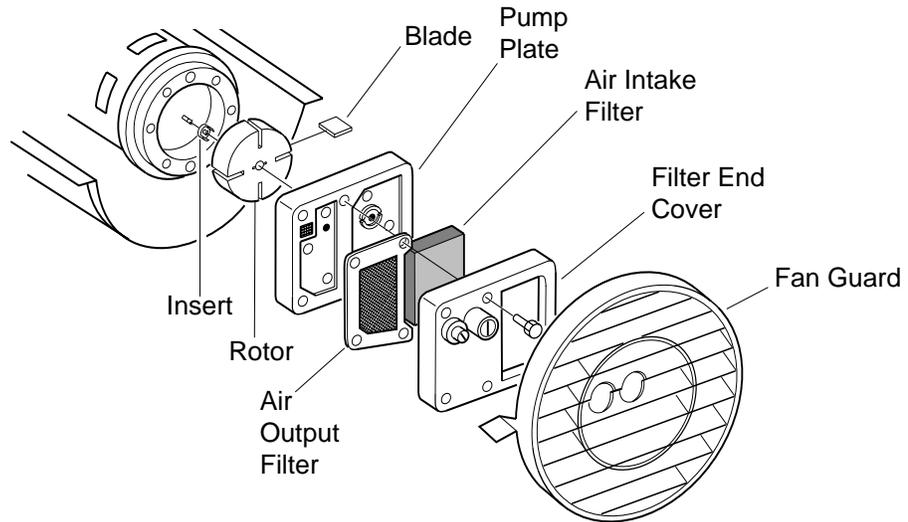
**Figure 15 - Rotor Location**
