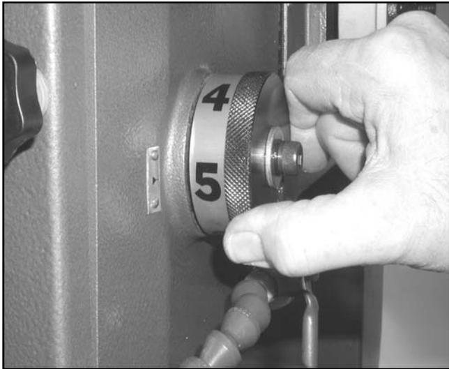
**Figure 19.** Depth control ring.
