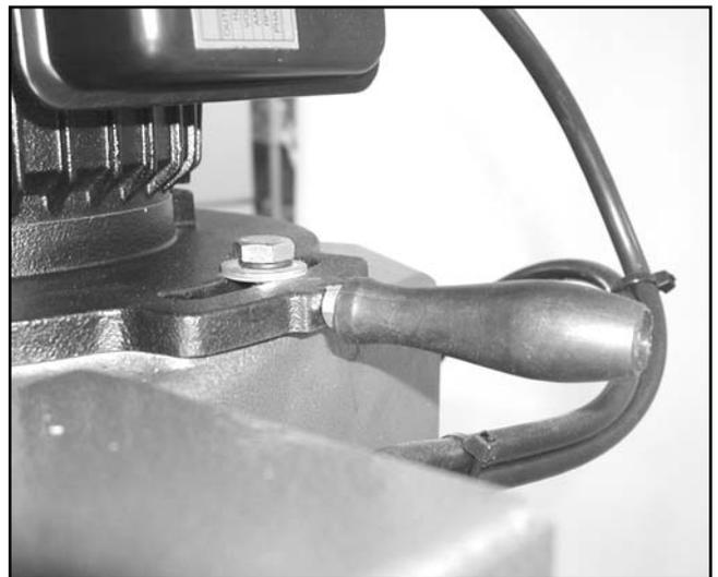
**Figure 14.** Belt adjustment handle.
