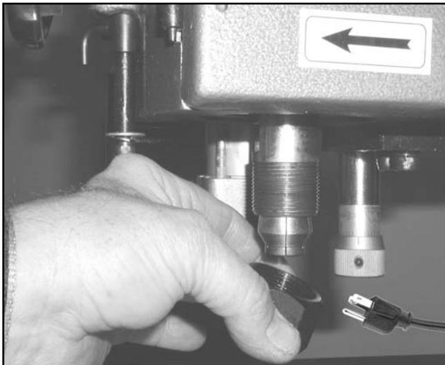
**Figure 7.** Installing collet nut.
