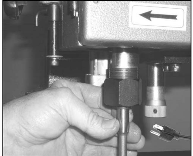
**Figure 8.** Installing the router bit.
