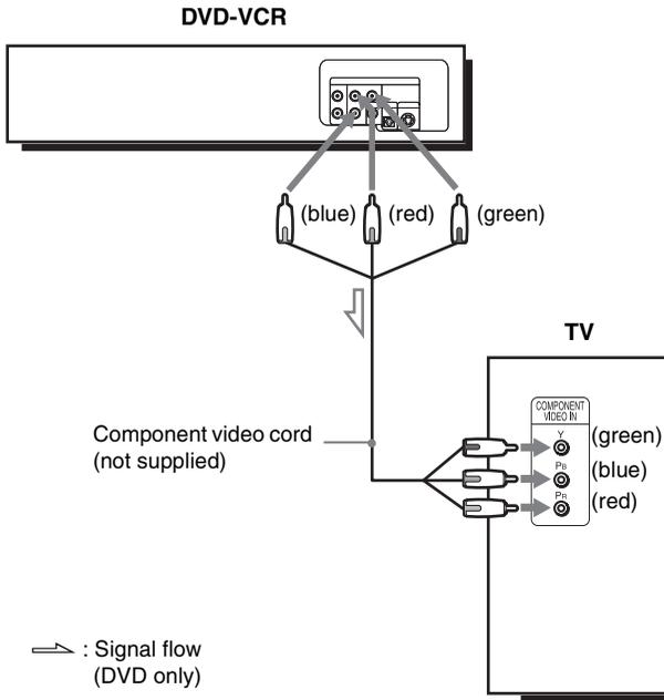
If your TV accepts progressive (480p) format signals, you must use this connection and then set “Progressive” to “On” in the “SCREEN SETUP” menu (page 57). The PROGRESSIVE indicator lights up in orange when the DVD player outputs progressive signals.
