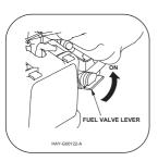
2. Turn the fuel valve lever to the ON position.
