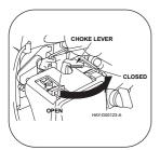
To start a cold engine, move the choke lever to the CLOSED position.
