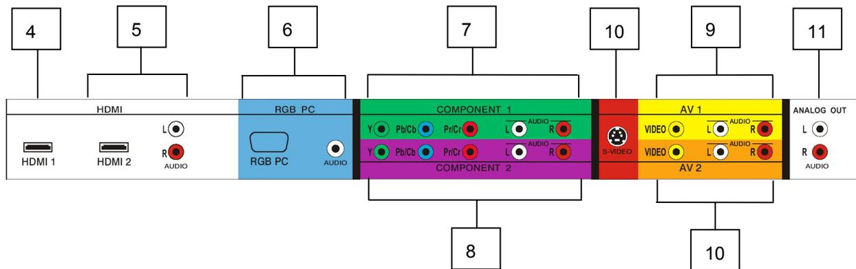
4. **HDMI 1** – Connect the primary source for digital video such as a DVD multimedia player or set top box through this all digital connector. The white color band on the rear of the TV indicates this connection. Your VIZIO Certified HDMI cables are available for purchase from [www.vizioce.com](http://www.vizioce.com) or by calling 888-VIZIOCE (888-849-4623).
