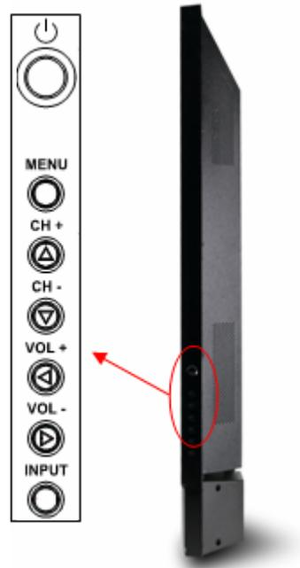
Additionally, when the OSD is active, this button confirms the menu function to be adjusted. When the OSD is not active, pressing this button will display the current input mode.
