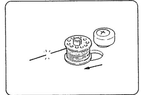
Wind thread until winder stops. Push bobbin winding spindle to the left and clip thread. Remove bobbin. Turn clutch knob away from you while holding hand wheel for normal sewing operation.
