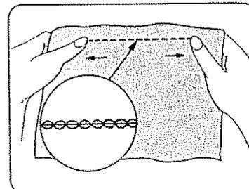
The stretch stitch does not actually stretch as it is being sewn, but is stitched in a forward and back motion (sometimes called a “reverse-action” stitch), so that it will give when the fabric stretches instead of breaking. This stitch can also be used for topstitching on all fabrics.
