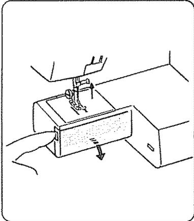
Remove the extension table from the machine by pulling it to the left. Open the shuttle cover by pulling down the embossed part on the left side of the cover.
