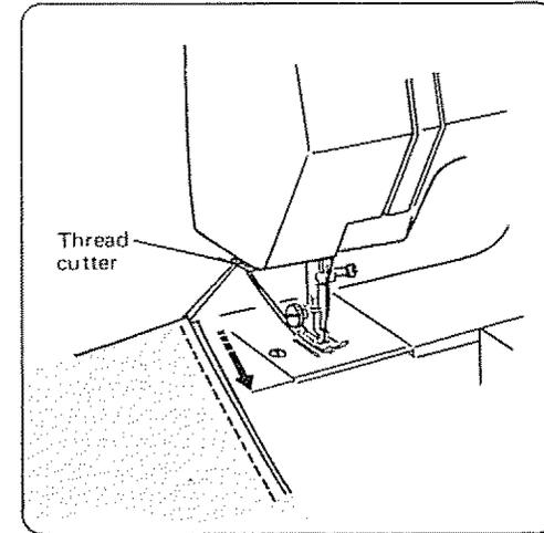
You don't need a pair of scissors to cut the thread after you finish sewing. Just use the handy thread cutter.
