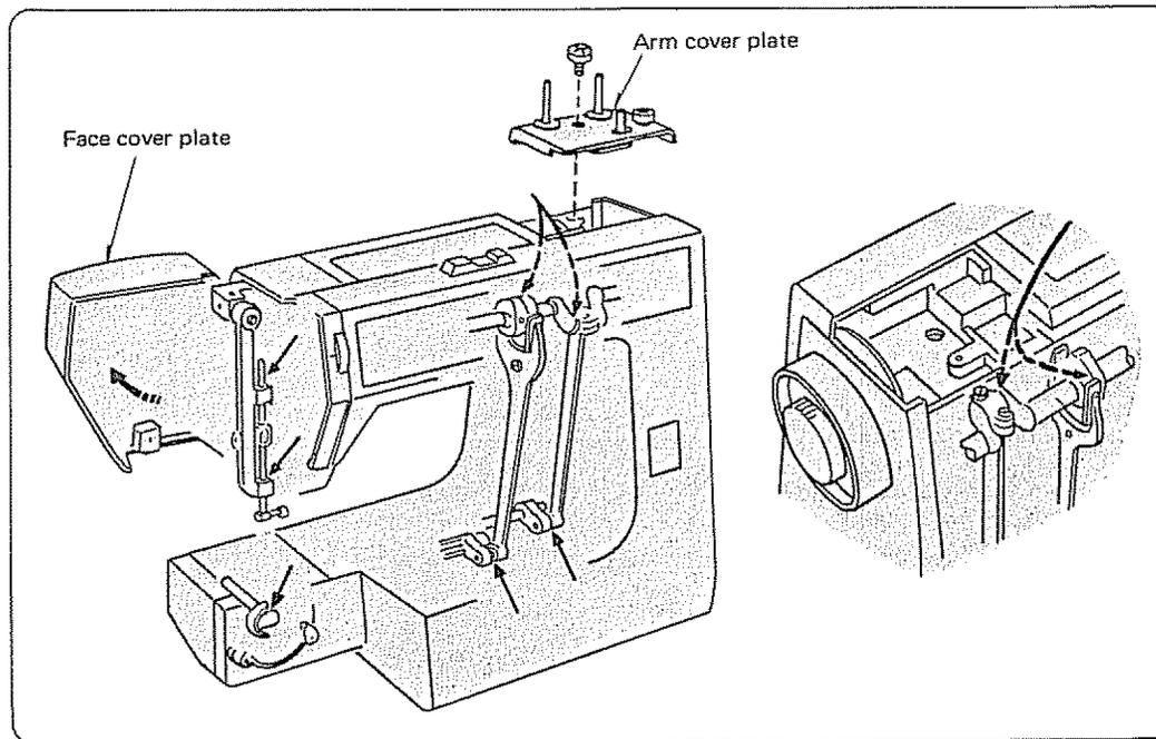
Open face cover plate and/or remove arm cover plate by loosening top screw to oil points in illustration.
