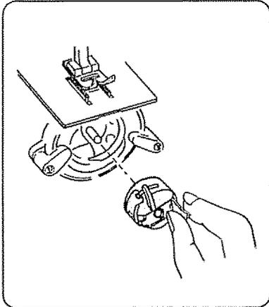
To remove bobbin case from shuttle, pull open latch of bobbin case. Pull bobbin case straight out of shuttle.
