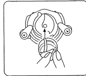
Holding latch open, position case into shuttle and release latch.
