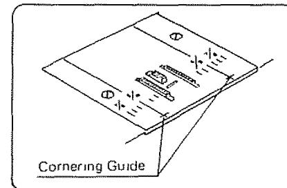
The seam guides on the needle plate are there to help you measure seam width. The lines are 1/8" apart, with the 5/8" and 7/8" lines marked.
