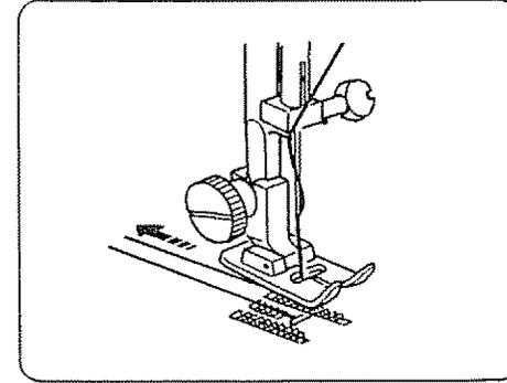
3. Pull both threads under and to the back of the presser foot, leaving 4 to 6 inches of thread clear.
