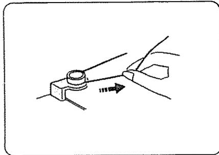
Draw thread from spool through bobbin winding tension disc as shown.
