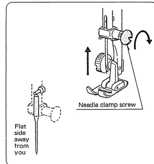
**NOTE:** Raise the needle bar to its highest position by turning the hand wheel toward you.
