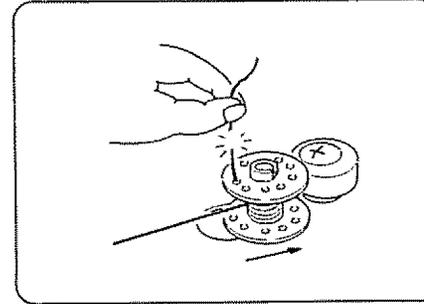
Place bobbin onto bobbin winding spindle with end of thread coming from the top of the bobbin. Push bobbin winding spindle to the right until it clicks. Holding onto end of thread, start machine. When bobbin is slightly filled, snip off end of thread.
