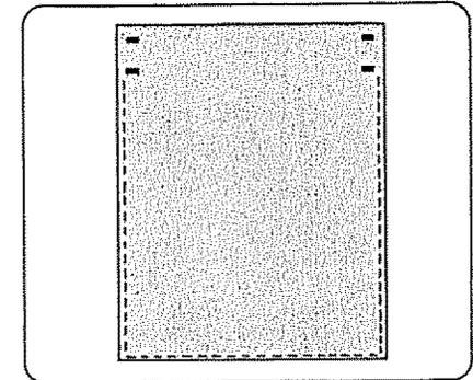
This stitch is similar to a very short satin stitch and is used to reinforce points of strain such as corners or pockets and straps on lingerie.
