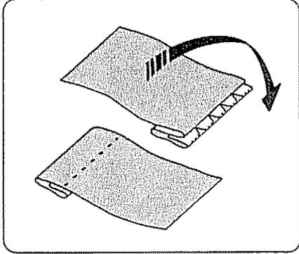
There are two blind hem stitches on your machine. The regular blind hem is used for woven fabrics. The stretch blind hem is wider and will "give" and is used for knit and stretch fabrics.
