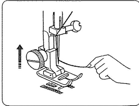
1. Raise presser foot lever. Hold top thread loosely in left hand and rotate handwheel toward you one complete turn.
