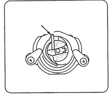
Case should lock into place when latch is released.
