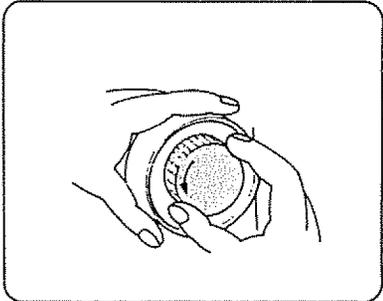
Release clutch by turning the clutch knob inside the hand wheel toward you to stop the needle from moving while you wind the bobbin.
