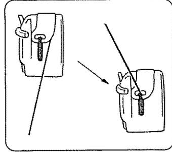
Pull thread under tension spring and through the opening as shown above. Pull 3 to 4 inches of thread from bobbin.
