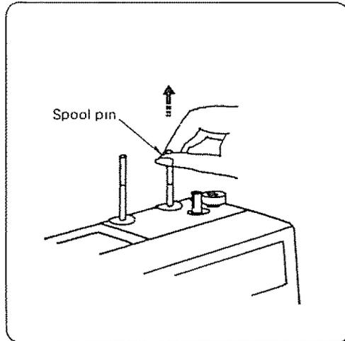
The spool pins are used for holding the spools of thread when feeding thread to the machine.
