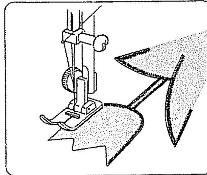
Baste (or fuse with iron-on fabric joiner) applique pieces on the fabric. Stitch around the applique making sure the needle falls along the outer edge of the applique.
