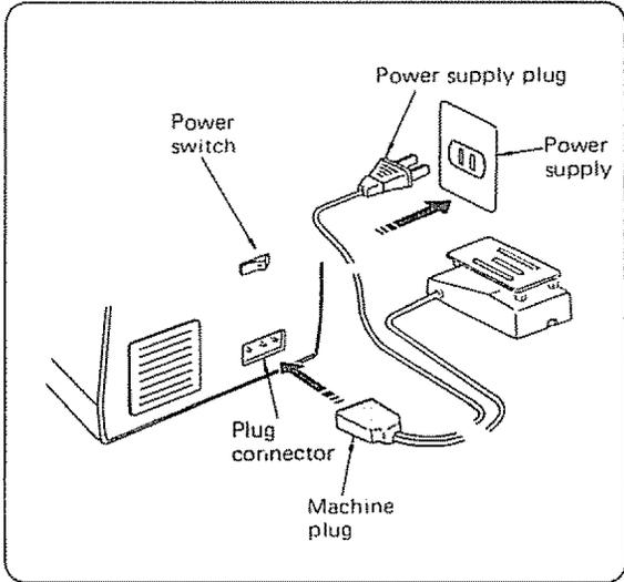
NOTE: Before inserting the plug into your machine, be sure the power switch is OFF.
