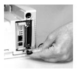
2 Attach the 10/100 Base-T UTP cable to the receptacle on the back of the OkiLAN 6120e. Attach the other end of the cable to the Network.
