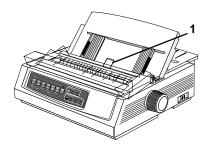
5 Adjust the paper feed guides (1) for the width of the paper. Place a sheet of paper in the separator. The paper will feed into the printer.
