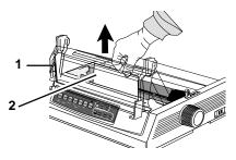
2 Remove the shipping restraint (1) behind the pull-up roller assembly.
