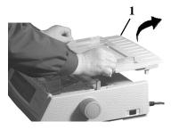
**4** Fold some continuous-form paper over three times to make a page four sheets thick. Then, load it on the tractors and close the covers.
