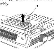
**3** Grasp the tabs and lift off the paper separator (1). Remove the shipping restraint (2).
