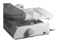
${\bf 8} \ \ \hbox{Install the pull-up roller assembly. Close the access cover.} \qquad {\bf 10} \ \hbox{Press FF/LOAD}.$
