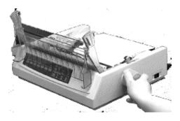
Load regular paper (making sure the tractor covers are closed). Install the paper separator.
