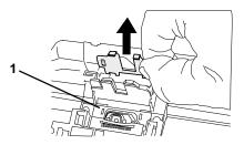
**8** Turn the printhead plate around and reinsert it on the other side of the carriage assembly (1).
