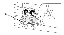
**9** Replace the printhead, making sure that the circuit board at the bottom of the printhead firmly engages the slot (1) in the carriage.
