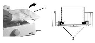
5 Install the paper separator. Install the pull-up roller assembly. Close the access cover.
