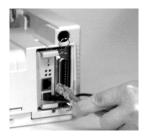
3 Plug the printer power cord into the power outlet.
