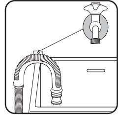
This could be done by tying it to the tap with a piece of string or attaching it to the wall.
