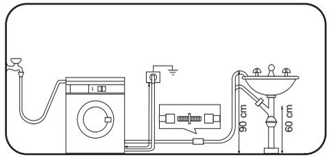
**For the correct functioning of the machine the drain hose must remain hooked on the proper support piece situated on the top part of back side of the appliance.**
