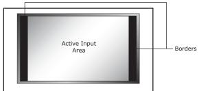
When the AAR is equal to the OAR (Output Aspect Ratio), the RS-VP2 supplies no border as shown below:
