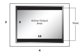
In this example, the region outside the Active Output area (called the mask) is inactive, and only important for creating video timing signals for the display. Input video data is never mapped to this region.
