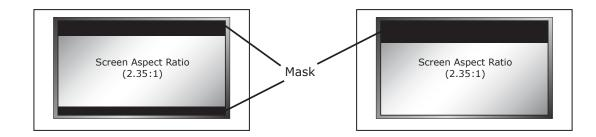
Underscan represents the visible display area, a sub-set of the Active Output Area. Underscan is like a negative zoom which preserves the aspect ratio of the active area. The default for this setting is 0. As you increase underscan, the smaller portion of the active display area appears while preserving the aspect ratio of the active display area. The Frame Geometry Test pattern should be used while making this adjustment.
