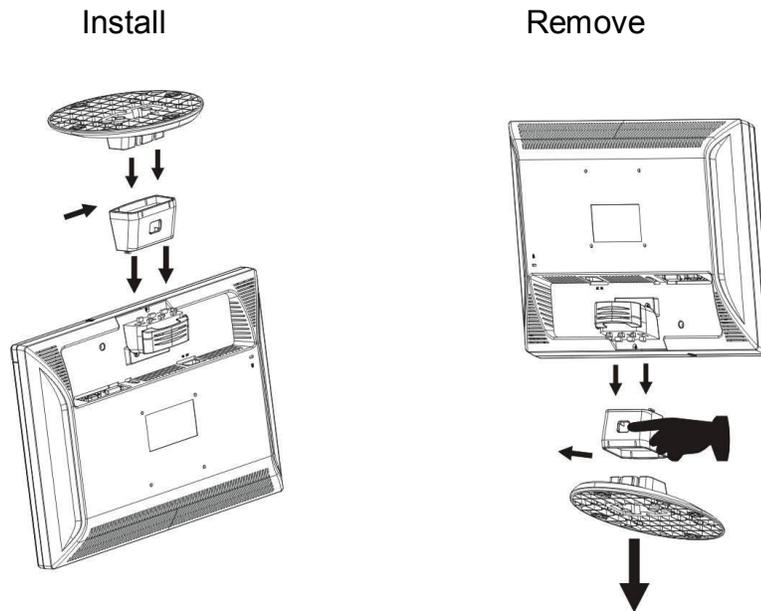
Figure 1 Installing and Removing the Swivel Base
