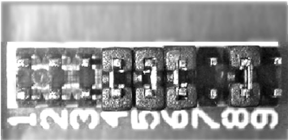
9 position jumper (This pushbutton is set for Ding Dong Chime since 7=off, 8=on, and 9=off.)
