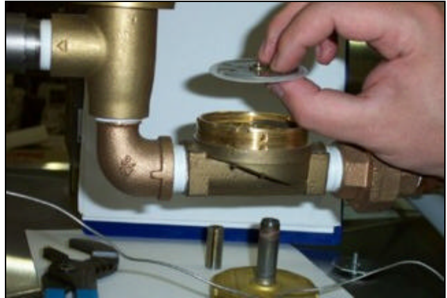
Removing the diaphragm
