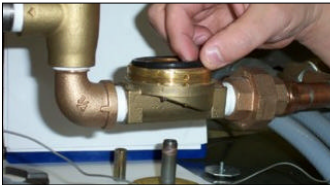
Removing the O-ring
