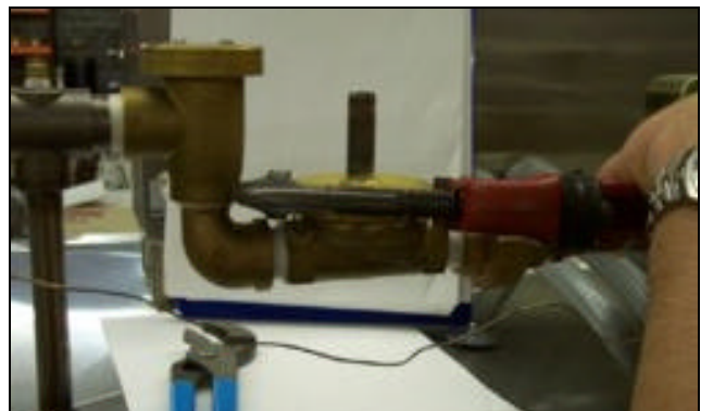
Loosening the valve bonnet
