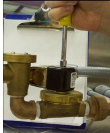
Removing the top screw
