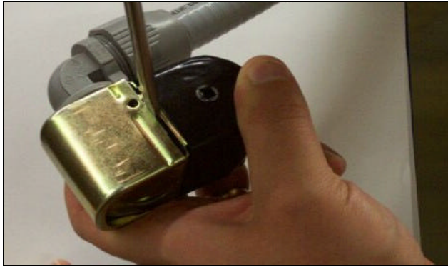
Prying open the coil wire cover
