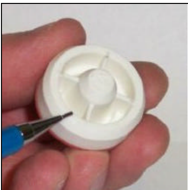
Examining the plunger seating surface
