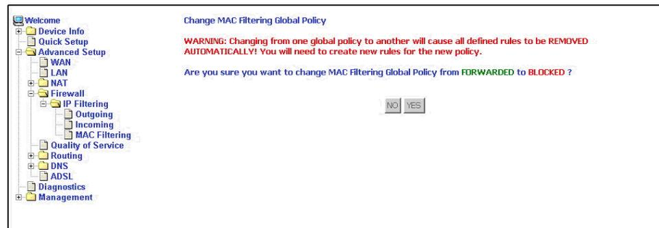
Figure 52: IP Filtering - MAC Filtering Policy Change Confirmation
