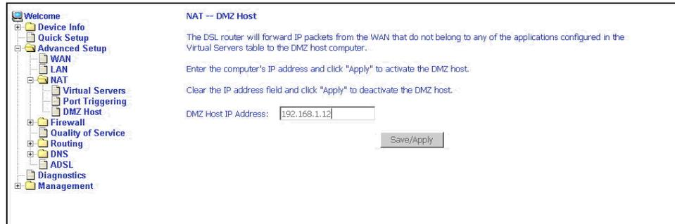
Figure 44: DMZ Host Setup
