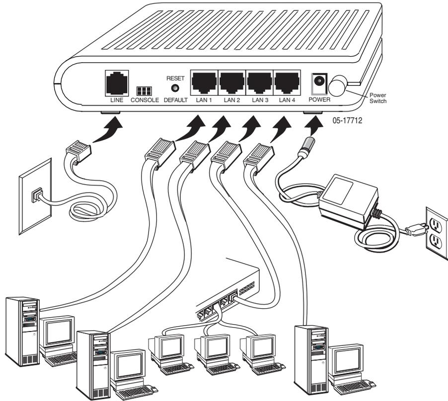
**Figure 3: Hardware Installation**
