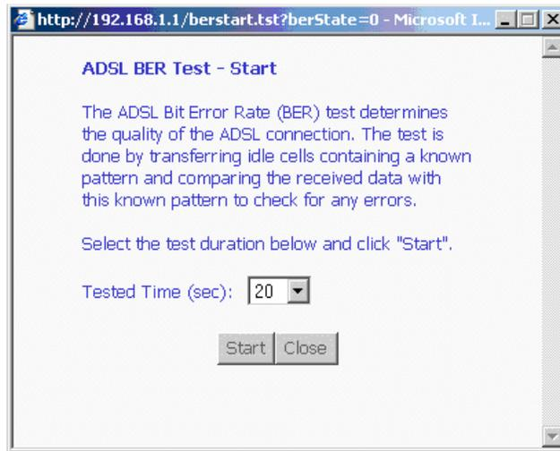
Figure 18: ADSL BER Test — Start
