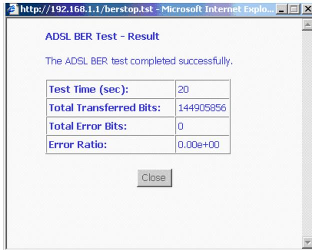
Figure 19: ADSL BER Test — Result
