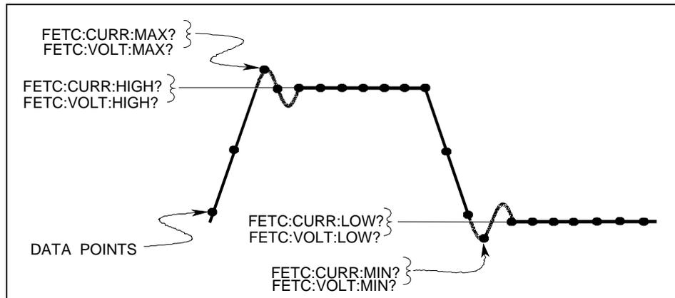
Figure 7-3. Measurement Commands Used to Return Pulse Data
