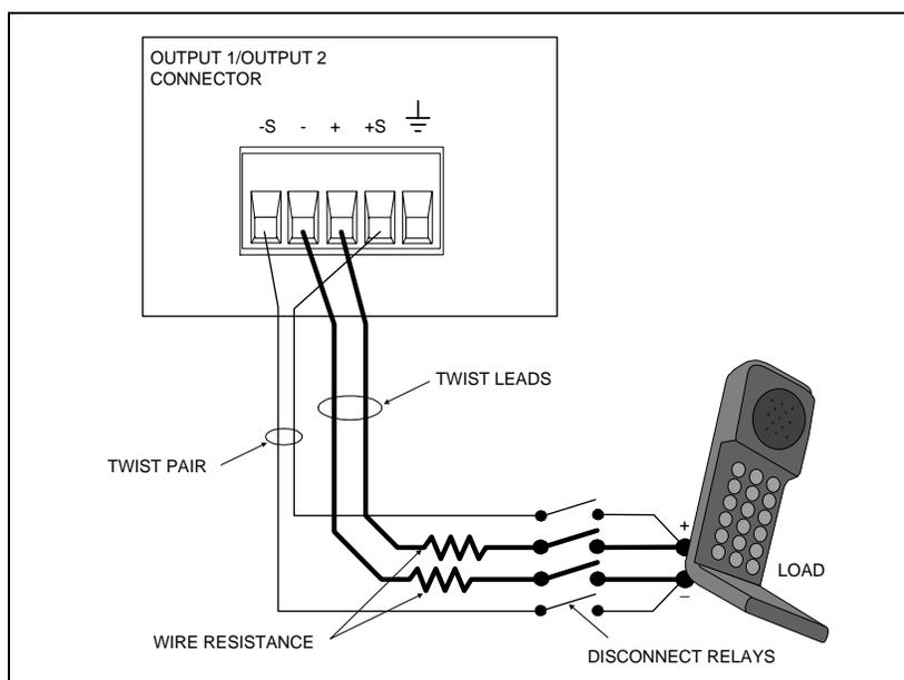
**Figure 3-3. Remote Sense Connections with External Relays**
