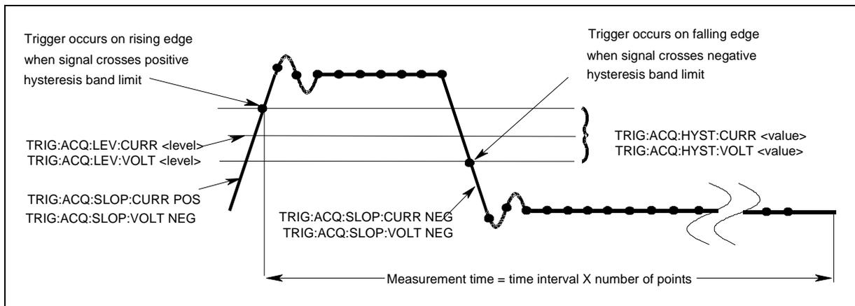
**Figure 7-5. Commands Used to Control Internal Measurement Triggers**
