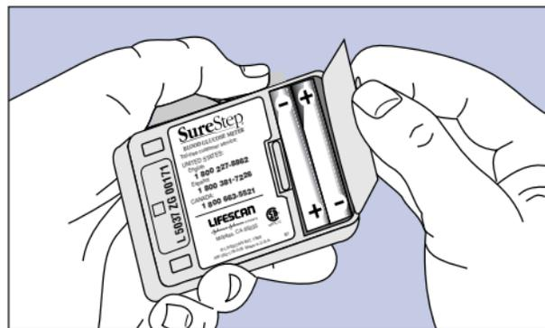
3. Remove the old batteries with your fingers, or by tapping the meter gently against the palm of your hand. Never tap the meter against a hard surface.
