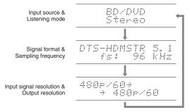
If "Dolby D 5.1" is displayed in Signal format, the Dolby Digital 5.1 ch signals are being input. When listening to AM/FM radio, the band, frequency and preset number are displayed.
