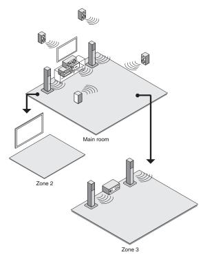
■ Types of source you can enjoy in a separate room: As the Zone 2 playback source, you can select from an external device connected to the HDMI input jack or the analog audio input jacks (\*) of the unit, the "NET", "USB" and "BLUETOOTH" sources, and the AM/FM broadcasting. As
