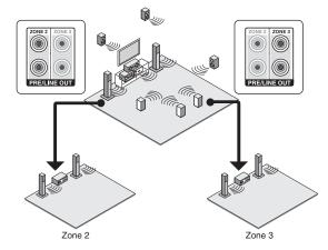
Volume can be adjusted with both the unit and the integrated amplifier used in a separate room. To adjust it with the unit, press RECEIVER and then HOME on the remote controller, select "Setup" - "7. Hardware Setup" - "Multi Zone" - "Zone 2 Out" or "Zone 3 Out" and set the setting to "Variable". If you connect a power amplifier, be sure to make the setting and adjust the volume in the main room.
