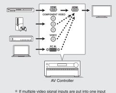
\* If multiple video signal inputs are put into one input system, the output will be made in the order of HDMI, component video, and composite video.
