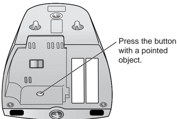
Pressing the FACTORY DEFAULT RESET button resets the camera to factory default. If you lose your user name and password, use this button to reset the camera. To restore the wireless connection, access the camera by using the wired connection and set up the wireless configuration. (See Getting Started.)
