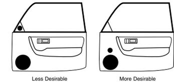
Avoid placing tweeters where they will be blocked by objects in the interior of the car (including seated occupants). When selecting a mounting location, look at both sides of the car to make sure that this location is clear on both sides.
