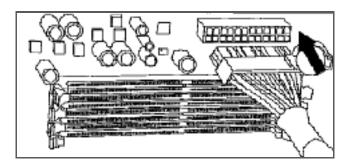
3. Connect the 8-pin (4 + 4) connector for the CPU.
