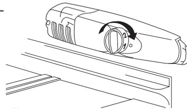
At a low ambient temperature of around 16°C, setting "1" should be selected. At ambient temperatures of around 25°C, select setting "2". If you require a lower temperature, select setting "3" or "4".
