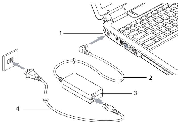
**Figure 3-1. Connecting the AC Adapter**
