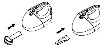
4. To use the flexible hose, push the smaller end of the hose into the suction hole, then attach the desired accessory to the other end of the flexible hose, as shown below.
