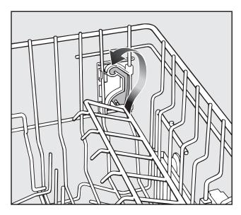
■ Pull the cup rack upwards and let it engage at the desired height.
