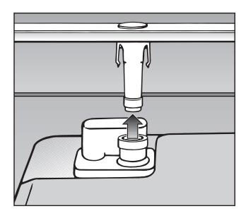
■ Pull the **lower** spray arm firmly upwards to remove.
