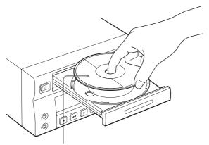
With the recording/playback surface facing down
