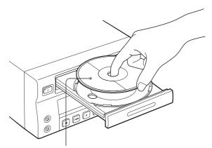
With the recording/playback surface facing down
