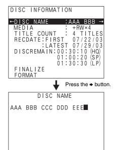
You can change the disc name on the above screen. However, you cannot edit the disc name on this unit. The RM-P110 (not supplied) is required. You can edit the disc name using the RM-P110 (not supplied) connected to the RS-232C connector. For detailed information on the RM-P110, see "To use an RM-P110 (not supplied) as a keyboard for editing/adding title name and information" on page 29.
