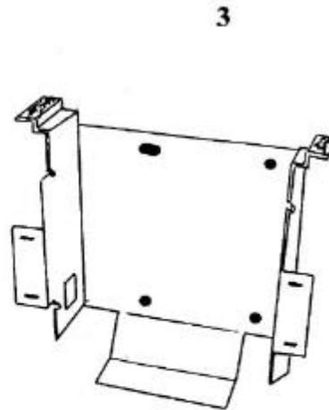
**REMOVE AND DISCARD (2) TWO SCREWS WHICH SECURE BRACKET TO HOUSING.**
