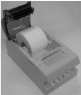
3. Drop the thermal paper roll inside the printer in the orientation as shown in the picture.
