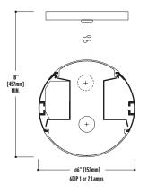
**Construction:** Extruded aluminum housing. Nominal 3', 4', 6' or 8' illuminated sections.
