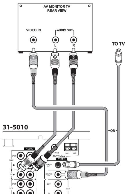
1. For audio, connect the plug from the TV's AUDIO OUT right jack to the receiver's right **AUDIO TV IN** jack and the plug from the TV's AUDIO OUT left jack to the receiver's left **AUDIO TV IN** jack.
