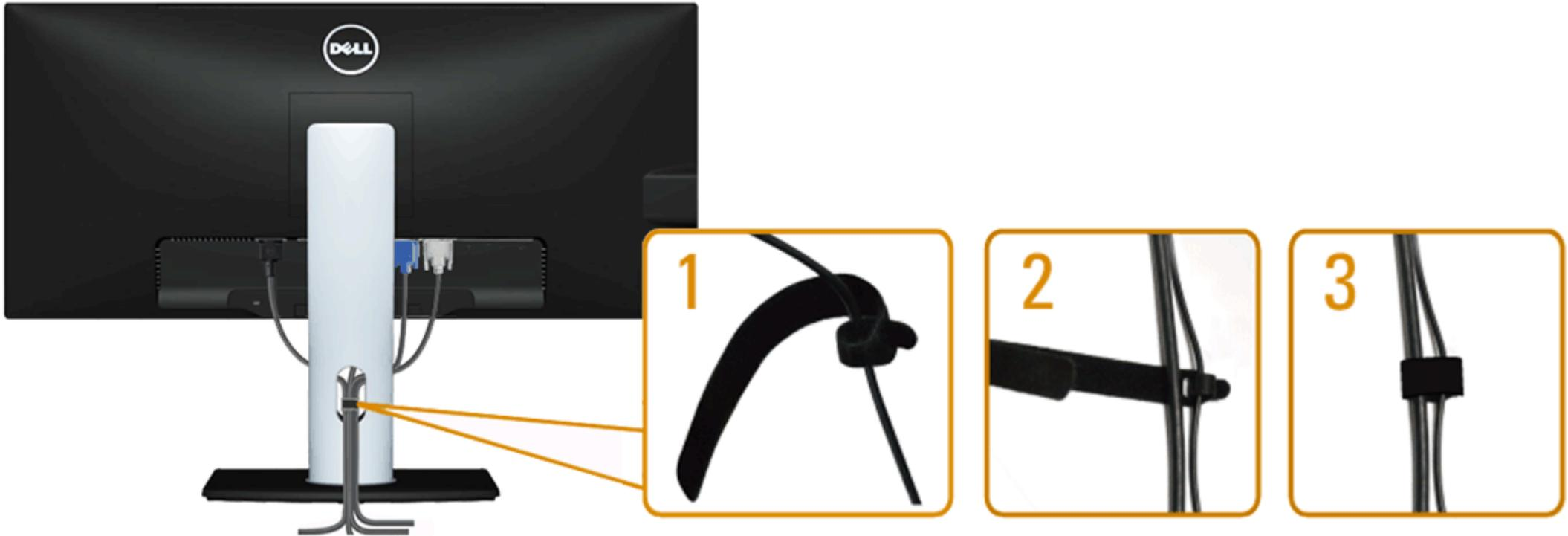
After attaching all necessary cables to your monitor and computer, (See [Connecting Your Monitor](#) for cable attachment,) use the Velcro cable tie to organize all cables as shown above.
