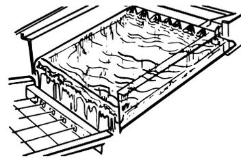
2. When the desired thickness is reached, the ice sheet is released and slides onto a cutter grid. The grid divides the sheet into individual cubes.
