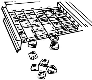
**NOTE:** As the room and water temperatures vary, so will the amount of ice produced and stored. This means that higher operating temperatures result in reduced ice production.
