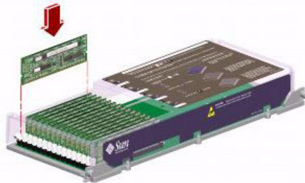
9. Push firmly and evenly on both ends of the memory module until the bottom edge is firmly seated in the socket. You will hear a click when the ejection levers are in the locked position.
