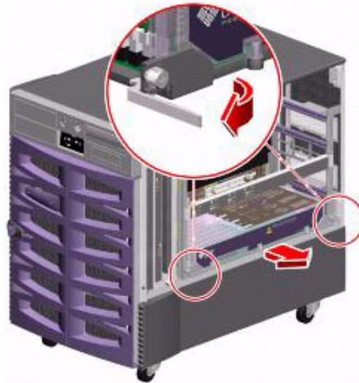
6. Pull the CPU/Memory board from the chassis.
