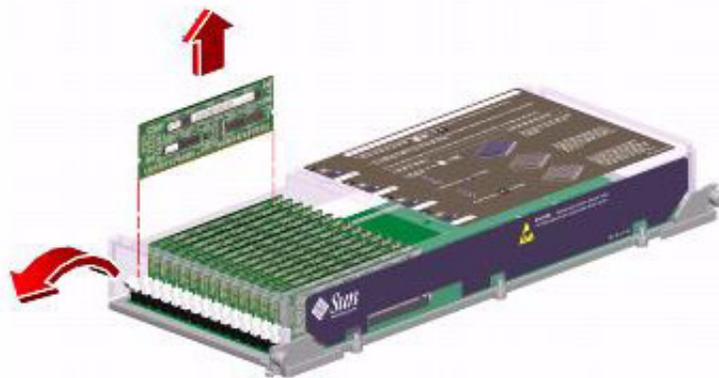
5. Grasp the top corners of the memory module and pull it up and out of the socket.
