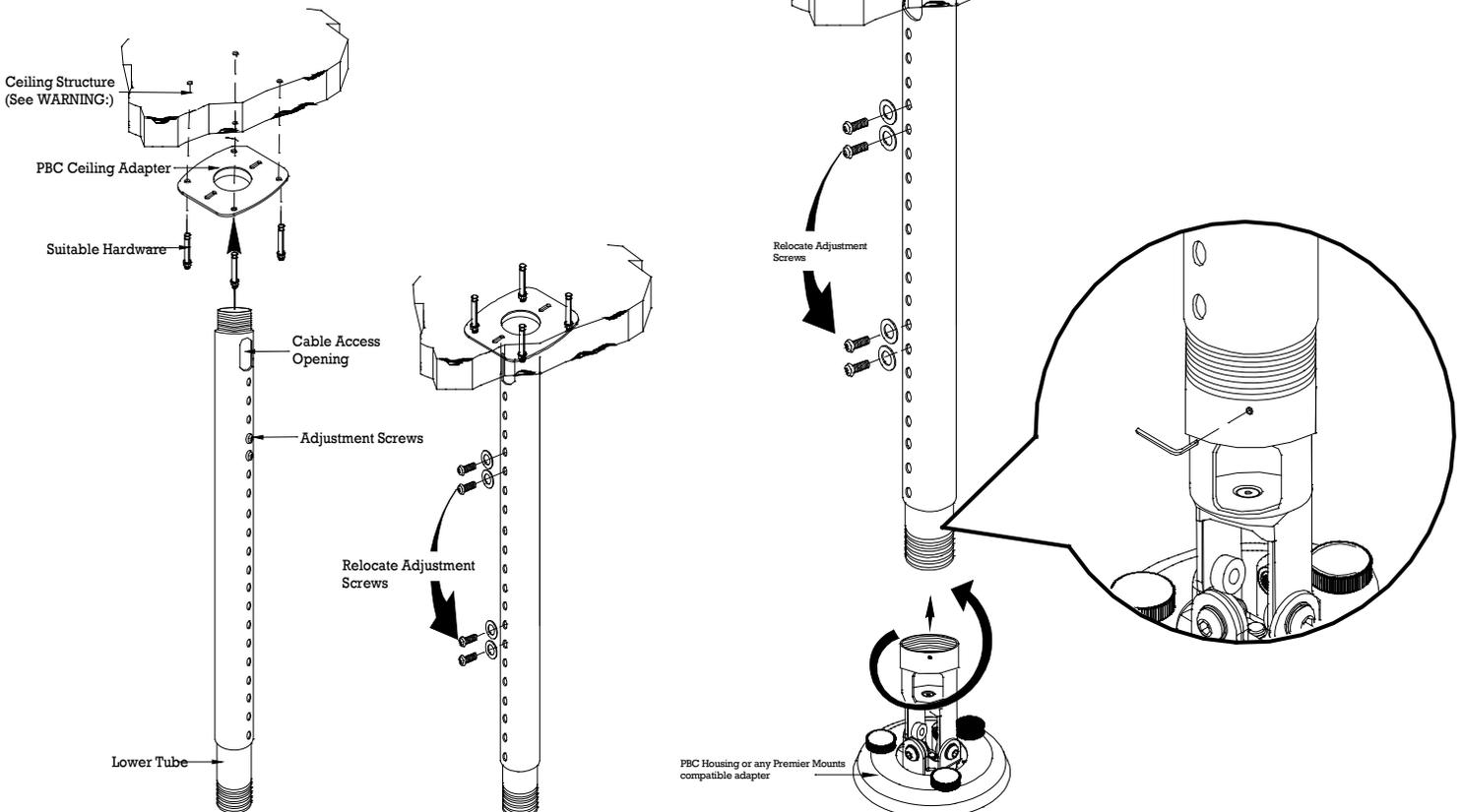
1. Secure the PBC ceiling plate or any 1-1/2 (NPT) pipe-receiving adapter to the ceiling (see warning).
