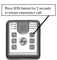
□ The device will send an alarm message and GPS coordinates to the Control Base. The Control Base software will find the street name and closest intersection from a map server and send these details through SMS short messages to all Contact numbers, with the text (example):
