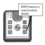
The device will collect GPS data (ca. 30-60 sec) and send a message and GPS coordinates to the Control Base. The Control Base software will find the street name and closest intersection from a map server and send these details through SMS short messages to all Contact numbers, with the text (example):
