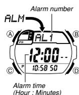
The Alarm Mode gives you a choice of four one-time alarms and one snooze alarm. Also use the Alarm Mode to turn the Hourly Time Signal (**ΣIG**) on and off.
