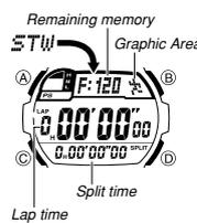
The 1/100-second stopwatch can measure elapsed time and lap/split times. Stopwatch times are stored in memory.
