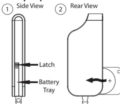
1. Using a small flat narrow object, push latch down towards battery tray while gently prying the tray outwards from both ends until released. Remove the tray from the remote control housing.
