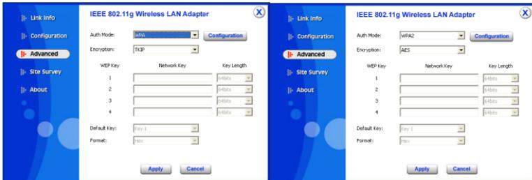
If WPA or WPA2 is selected, the above screen is shown. Please select the encryption type from drop down menu and press Configuration button to configure parameters for the RADIUS server.
