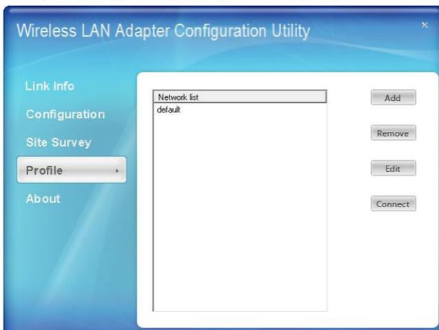
**Add:** Adds a profile. The following screen will appear. The user can enter the necessary information required for accessing Access Points or Wireless Router.
