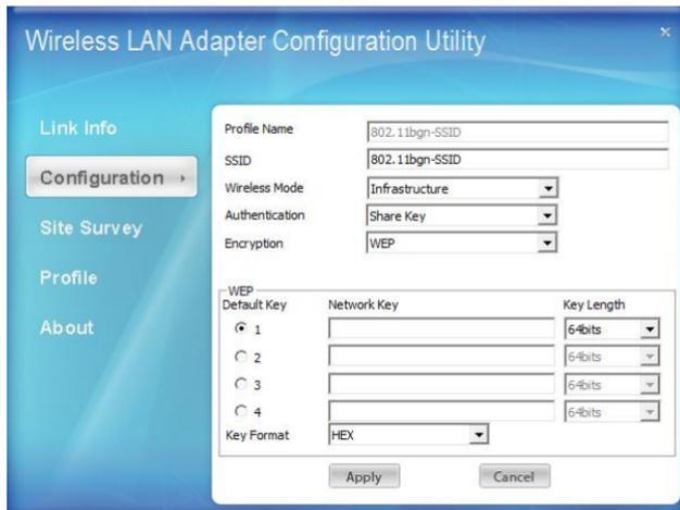
**Profile Name:** The default name is the same as the SSID of the platform which you connected and you can change the name you favor( the key length is limited 1~32 bits).
