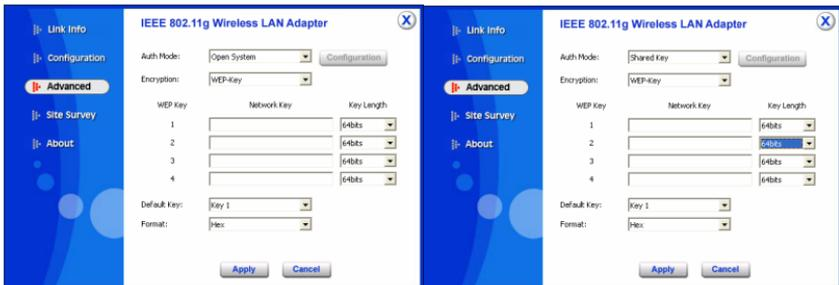
**WEP Key 1~4:** choose the encryption way, either in HEX or ASCII formats, and enter the password in the blank space.
