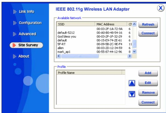
**Available Network:** displays the wireless networks (wireless clients and Access Points) that are in signal range.
