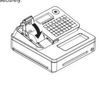
Note: Never touch the printer's thermal head and the platen. Avoid the thermal paper from heat, humidity or direct sunlight.
