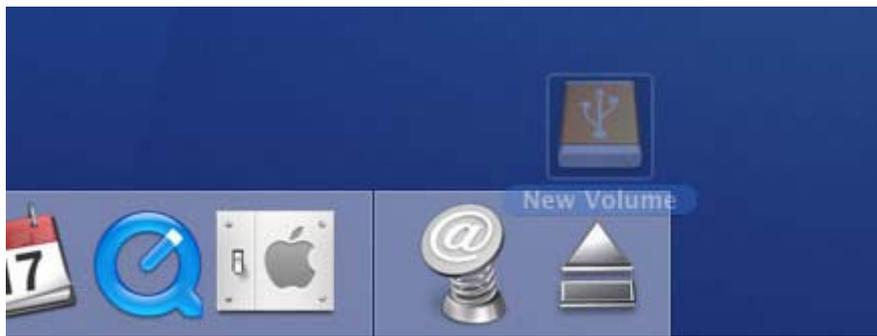
Figure 7: Drag StoreJet 25 drive icon into the Trashcan
