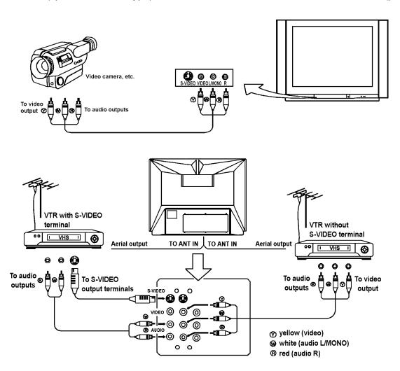
To select the input press the AV button on the remote controller repeatedly until you see the corresponding input indication on the screen. To return to aerial input, press the AV button until it displays programme number, or press direct channel select button or the CH  $\triangle / \nabla$  button.
