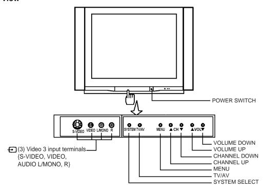
Note: Functions of MENU, TV/AV, SYSTEM, VOL ▲/▼, CH ▲/▼ are also provided to the remote controller.
