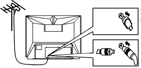
Note: In case of using the Twin-lead aerial feeder ( $300\Omega$ ) for UHF/VHF aerial, use a 300-75 ohm adaptor (not supplied)
